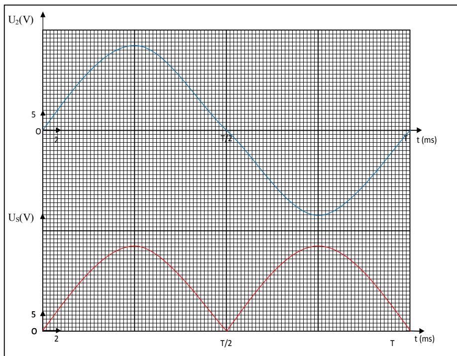
3)  $U_{S\text{moy}} = 2U_{S\text{max}}/\pi = 13,47 \text{ V}$ ;  $U_{S\text{ef}} = 15 \text{ V}$  ..... 2pts (1pt chacune)
